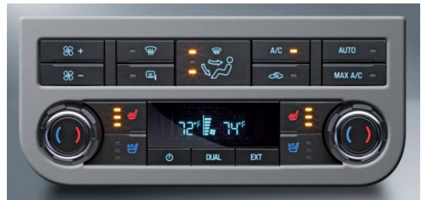
Figure B2: The control panel for a climate control unit
